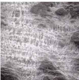
SINBRAN® filter surface filtration, smooth surface, fine texture
