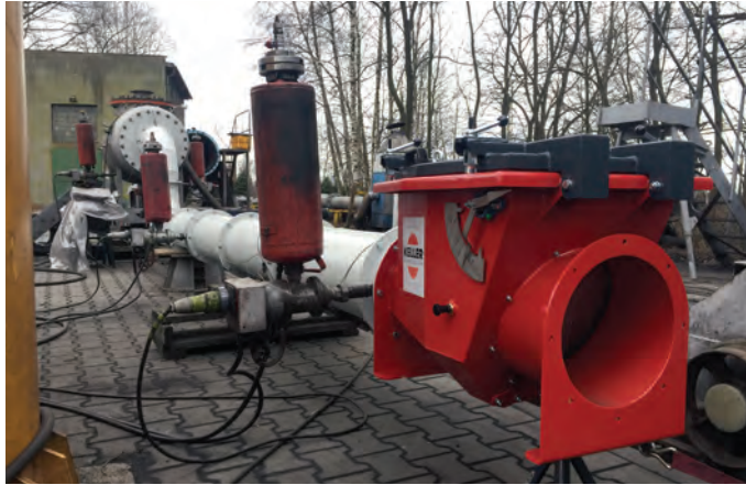
Back pressure flaps must comply with the stricter test standard (EN 16447). The new Keller ProFlapIII series successfully granted approval.
