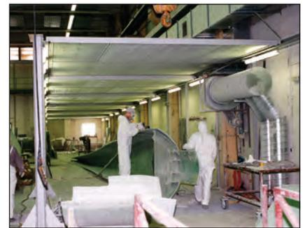
Soundproofing cabin with integrated collection and filtering system. Application: Grinding of FGRP materials (rotor blades).
