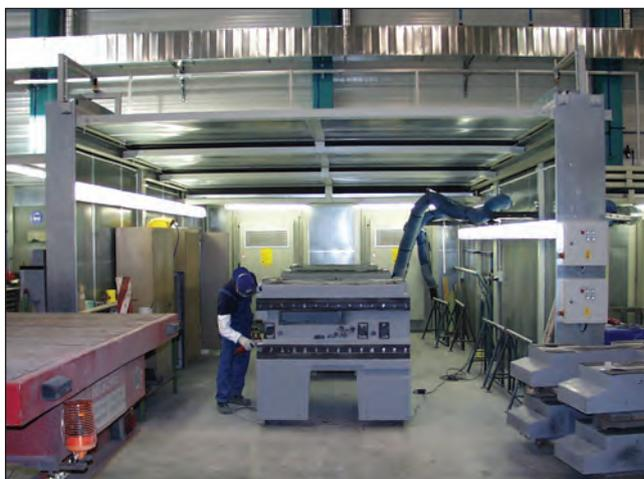
Soundproofing cabin with integrated collection and filtering systems
