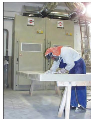
Pneumatic removal and filtering during grinding of FGRP materials.
