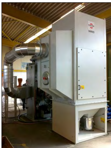
Dry separator VARIO especially developed for spring end grinding
