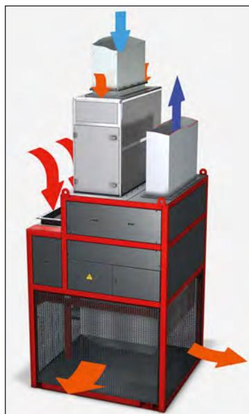
Example A: The cleaned exhaust air and the outdoor air are heated on demand and combined with ambient air inside the plant.
