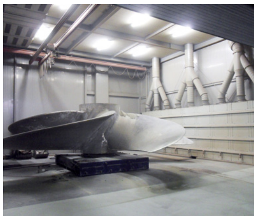
The air to be separated is extracted rapidly through slots in the wall.
