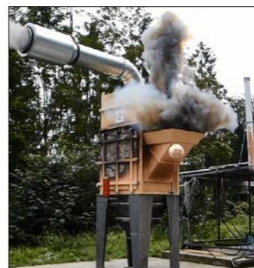
Explosion suppressed by ProPipePlus
