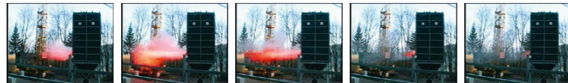
Testing the explosion potential of filter housing at the FSA facilities
