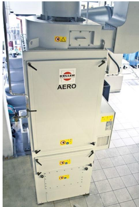
Three Keller extraction systems operate at Emil Arnold. One of the units, the oil mist separator AERO, filters 99 percent of even the finest aerosols from the air.
